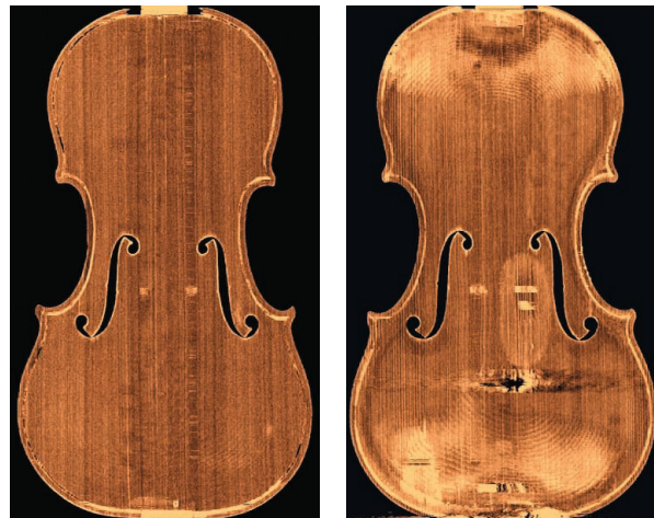
Like new. Typical patches and repairs show up as light spots in the CT scan of a 1730s violin (right). The Vieuxtemps (center) is spotless.
